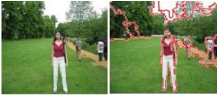
Fig 9: Example result of outdoor scene image segmentation using background recognition and perceptual organization. Adapted from [16]
